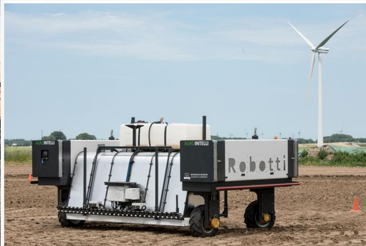
Wageningen researchers are developing a spot sprayer to combat, for example, volunteer potatoes in onions and beets. This in collaboration with a Robotti 150D field robot. Tests show that the spraying system needs to be even more robust.
