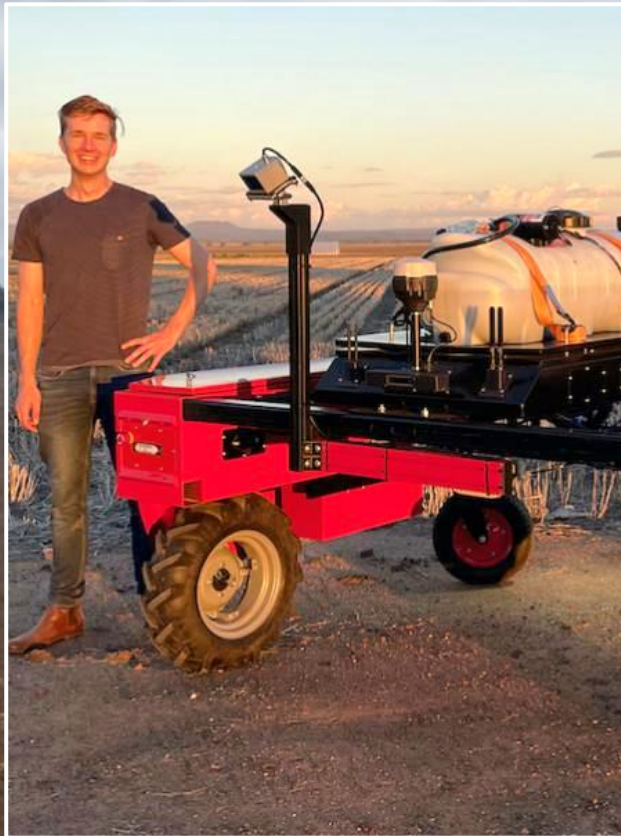
Wageningen researchers are developing a spot sprayer to combat, for example, volunteer potatoes in onions and beets. This in collaboration with a Robotti 150D field robot. Tests show that the spraying system needs to be even more robust.
