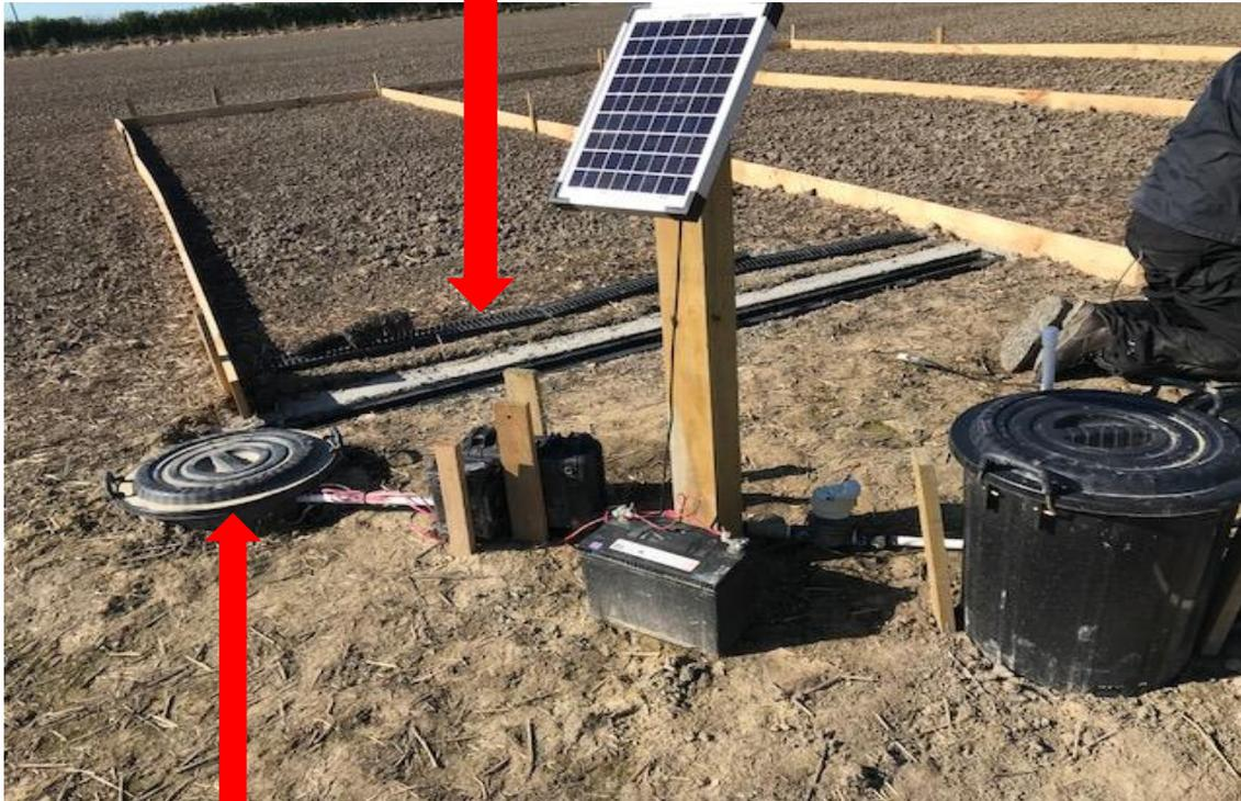
Water that ends up in the gutter gets channelled into the primary settling bucket (PSB).
