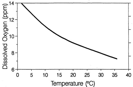
**Figure 2. The saturation level of dissolved oxygen at various temperatures (after Wilcox, 1980).**
