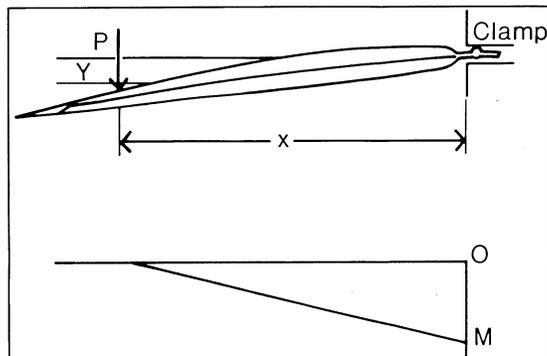
Figure 2. (b) Details of loading of the silique in evaluating shatter resistance of *Brassica*.
