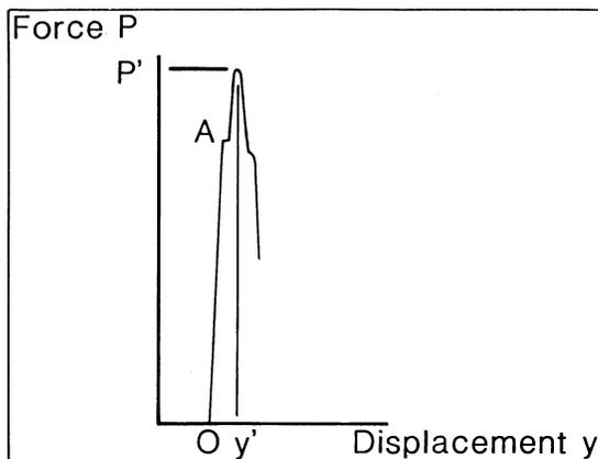
Figure 3. Force-displacement graph of a silique of *Brassica napus* before and after dehiscence in the testing machine.
