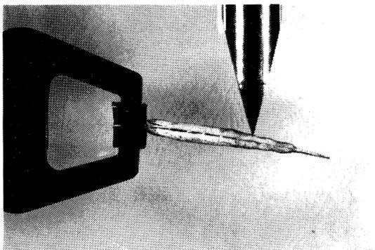
Figure 2. (a) Silique on dehiscence in the machine for measuring shatter resistance.
